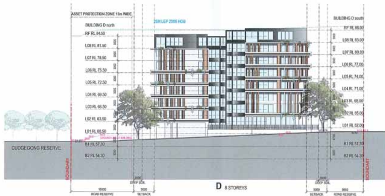
BUILDING E WEST ELEVATION
