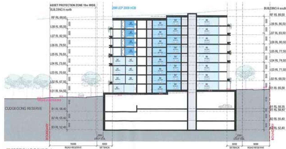
SECTION E-E BUILD A
